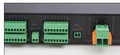
Connections Connections Quick coupling wiring terminal board.
